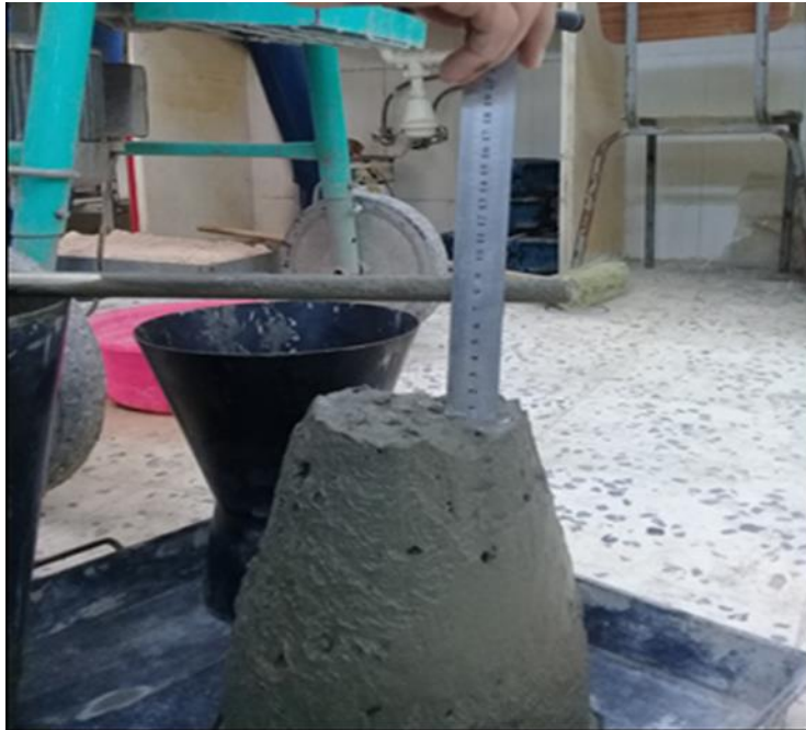
Figure 6: The slump test according to [BS 1881 part 116].
